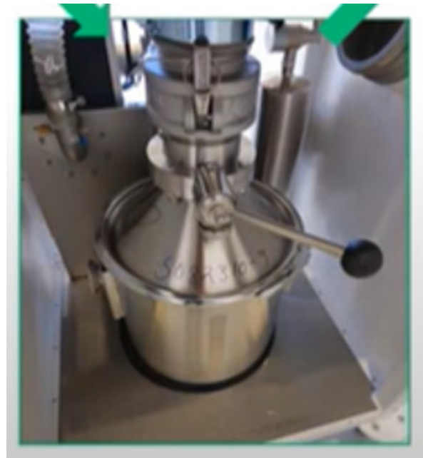
Figure 9. Identification number of the powder batch visible on the lid of the material container. (Image: AMEXCI Oy)
