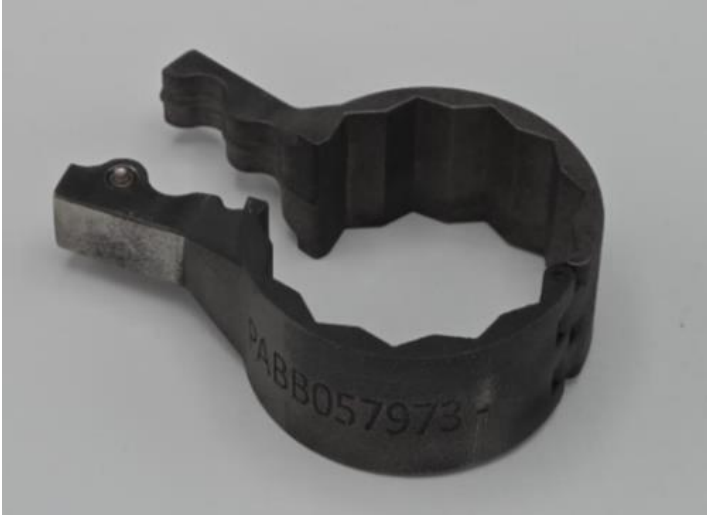
Figure 1. Tested wrench tool 3D printed of MS1 maraging steel.
